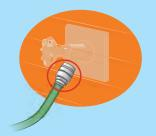
Protect your home with air vacuum breakers. Over half of the Nation's cross-connections involve unprotected garden hoses. Check to see if you have air vacuum breakers installed on each of your hose bibs. They prevent water from getting back into the drinking water system. These sample devices are inexpensive and can be purchased from your local hardware store. They are easy to install, you just simply screw them onto the hose bib.
